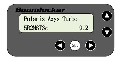
There are five buttons used to navigate through the Boondocker Control box.
