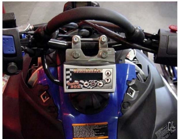
If the box is mounted under the hood, keep the box away from excess heat, including radiant heat. Also keep the box away from the ignition coils.
