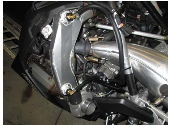
30. The Water to Air Intercooler system is now installed. Ensure coolant level is within range as indicated on bottle throughout use.
