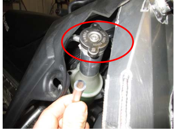
26. Add coolant to bottle. Make sure fluid level remains above the hose outlet on the bottle that connects to the turbo and pump.
