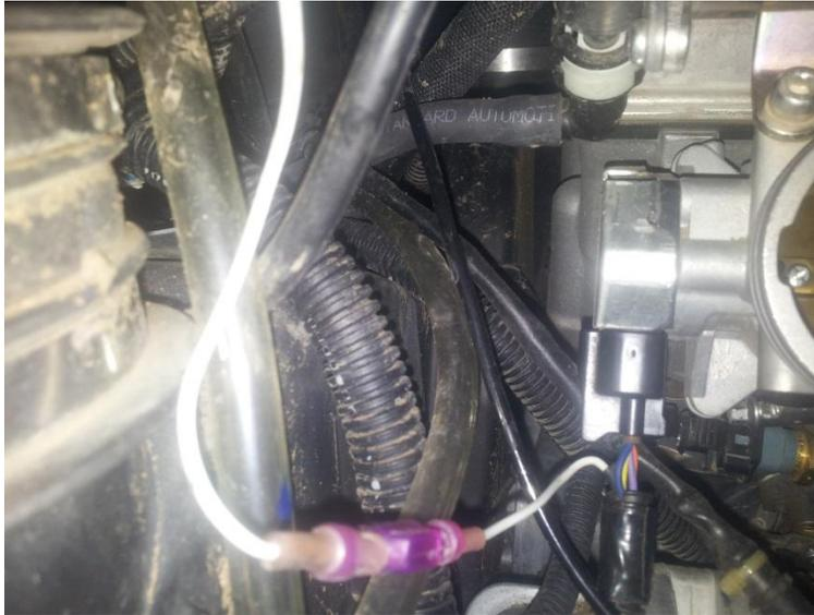
3. Tap the White wire to the Green Wire on TPS connector using supplied Heat Shrink Butt Connector. Shrink the ends using a heat gun.
