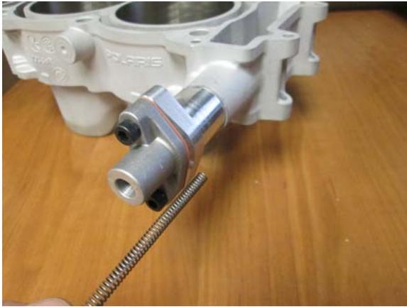
7. Before installing the tensioner spring assembly, check that all timing components are placed and correctly in time, then insert a small screw driver into the hole to push the plunger shaft making sure the plunger moves freely.
