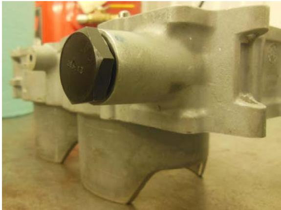
1. Locate and remove the stock timing chain tensioner on the MAG side of the cylinder.
