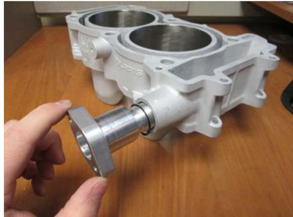
2. Place the included washer between cylinder and tensioner body, then screw the tensioner body clockwise keeping O-ring centered.
