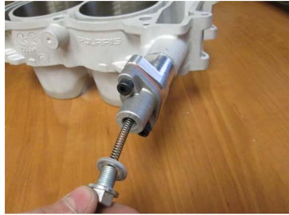
8. Install the tensioner spring assembly into the tensioner body and torque to 12 ft-lb.
