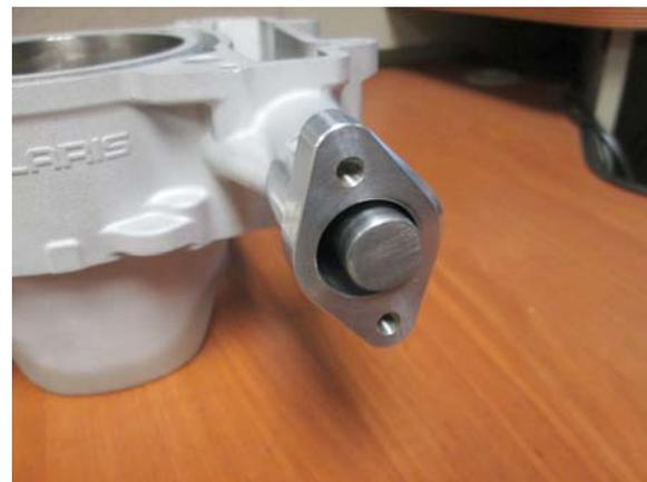
4. Cover the plunger with engine oil then push into the tensioner body as shown.
