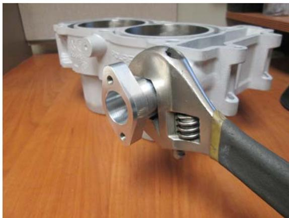
3. Use a wrench to tighten the housing until it is snug against cylinder (Do not over tighten).
